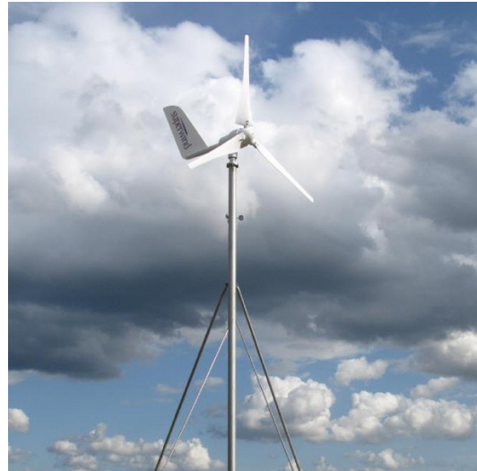
Figure 80: 1.25kW wind turbine 54
