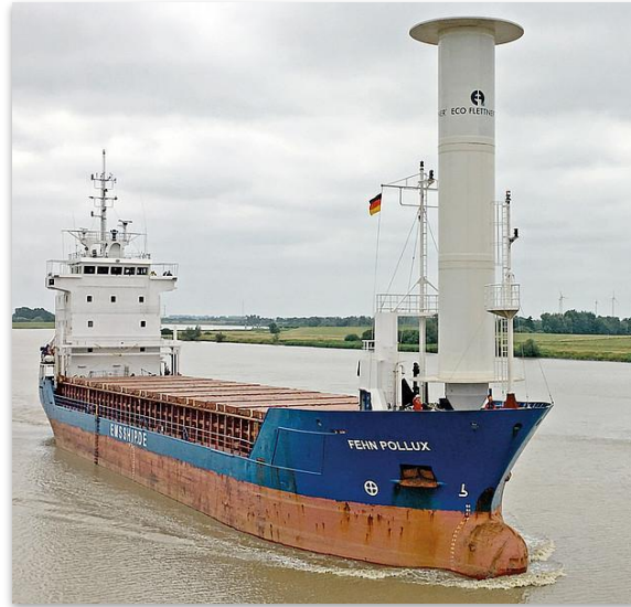
Figure 48: Cargo ship Fehn Pollux with Flettner rotor installation 40
