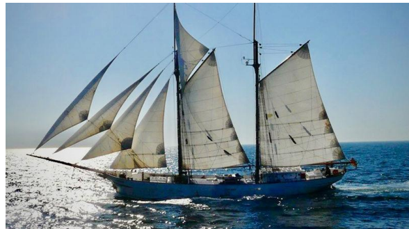
Figure 40: Sail cargo ship Kwai with a ketch type traditional rig, tripod mast, (left) 36 ; Sail cargo ship Avontuur, schooner type traditional rig (right) 37
