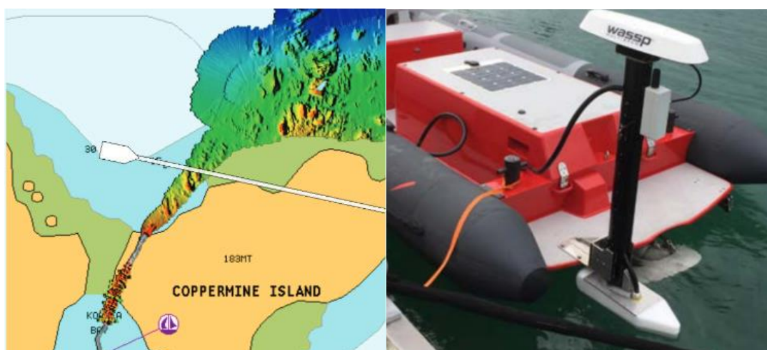
Figure 32: Survey data overlay (left) and WASSP S3 example installation on a RIB (right) 26
