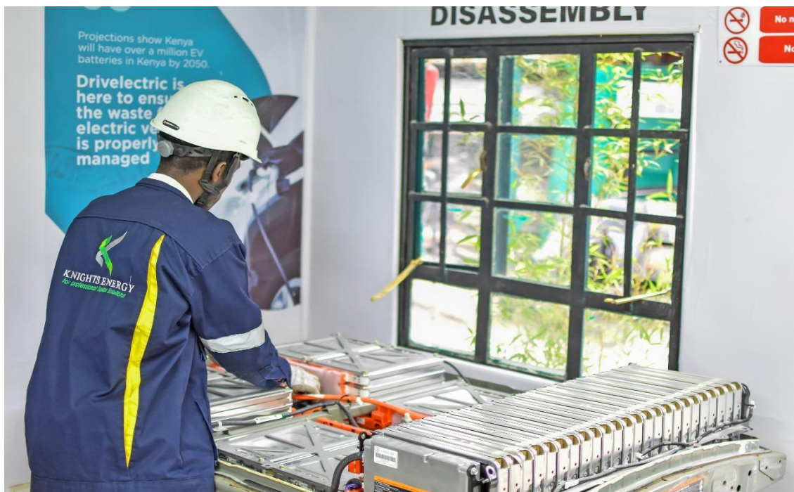
Figure 3 Knights Energy Engineer Disassembling a Nissan Leaf Battery Pack
