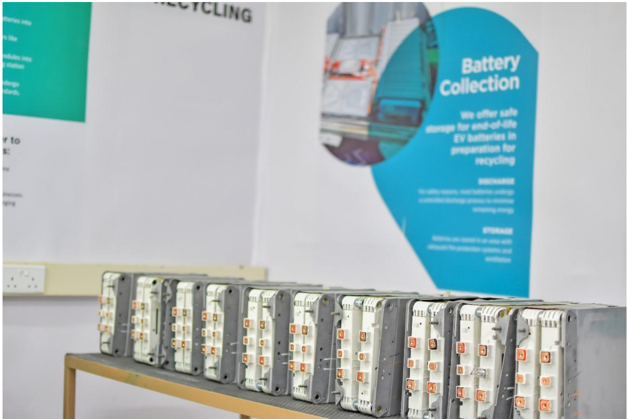
Figure 14 EV Batteries Preparation for Recycling
