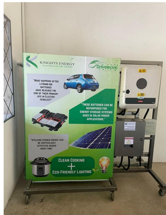
Figure 1 The Setup of the 7.77 kWh Battery from a Nissan Leaf Battery
