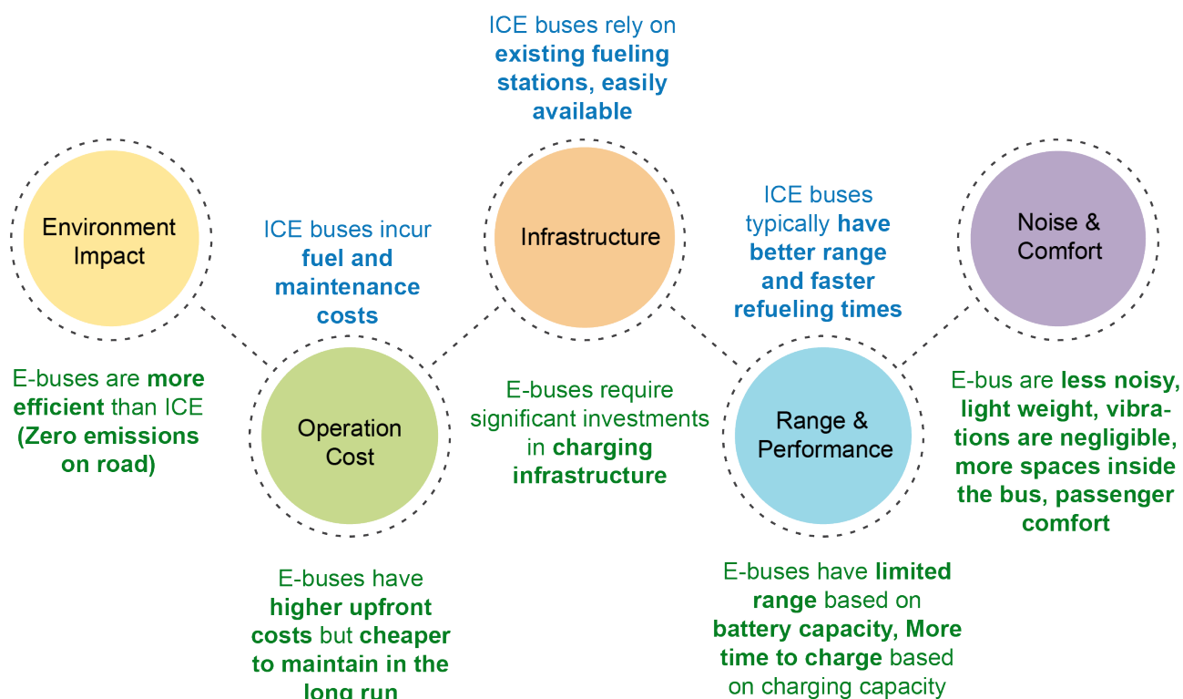
Figure 5.1: Difference in e-bus and ICE bus
