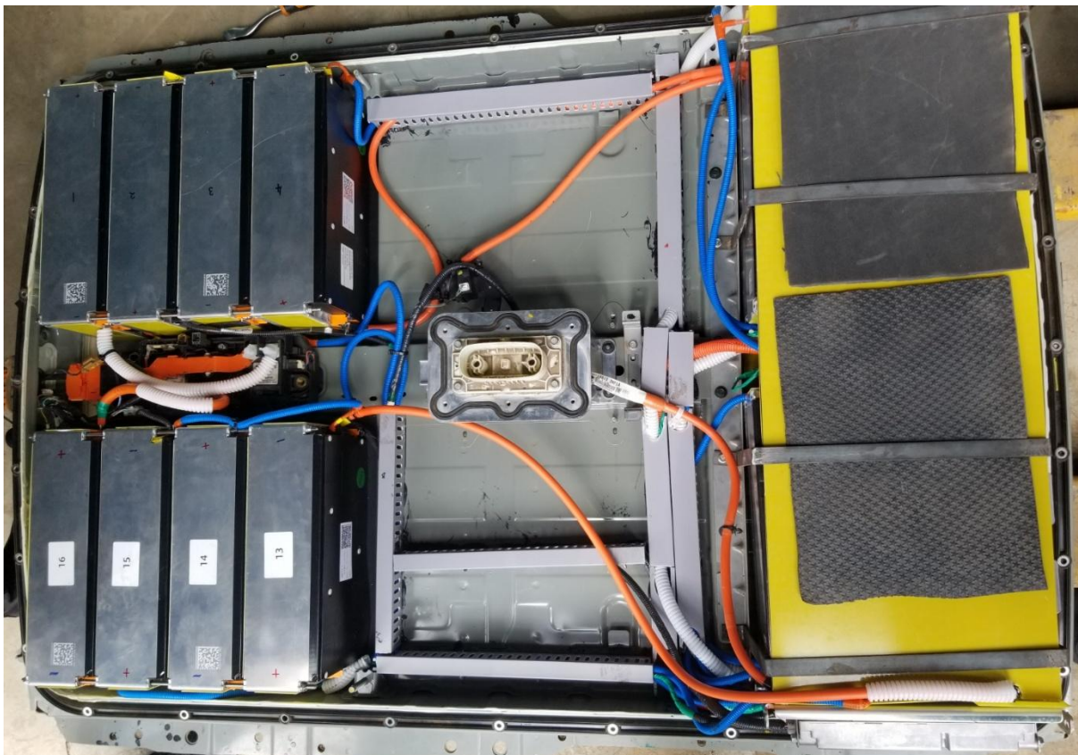
Figure 12 Final Assembled Battery Pack with Rear Modules Secure
