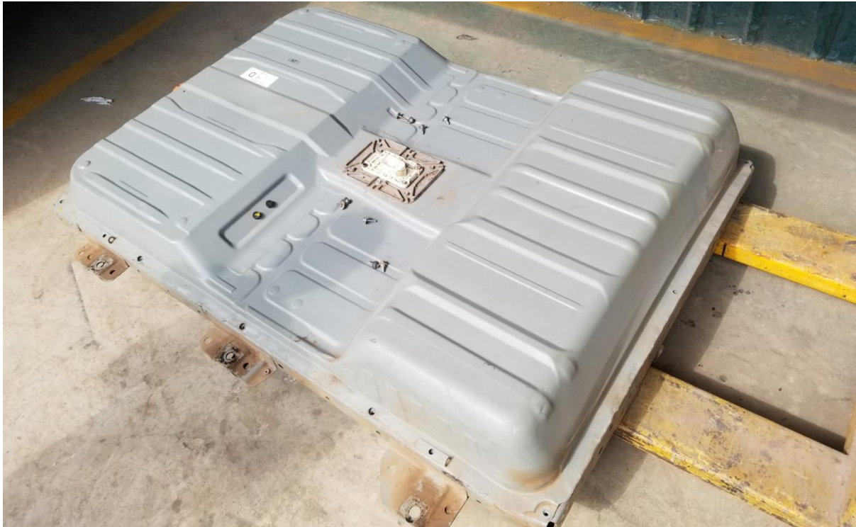
Figure 10 Original 24 kWh Battery Removed
