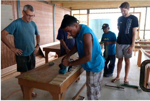
(a) Cut scarf bevels into plywood strips for beams using a planer.
