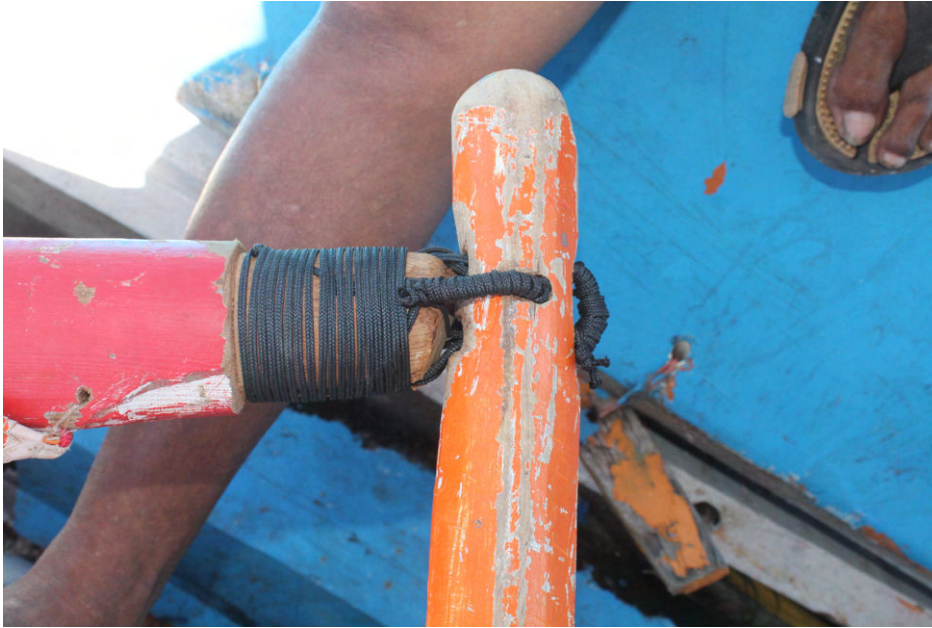
Figure 87: Lashing of the spar front ends ( kapelpel )
