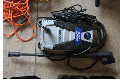
(b) High pressure cleaner (handy to clean dust off glassed hulls, but not really necessary)
