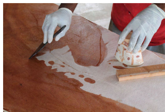
(b) Rinsing glass fiber cloth with epoxy resin to make GRP
