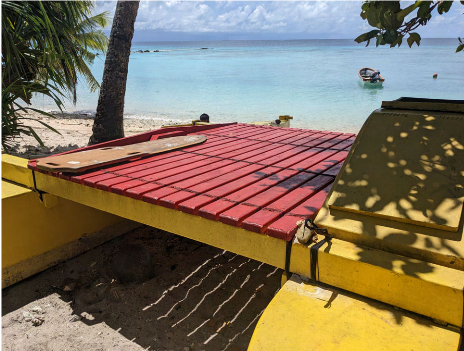
Figure 84: Slat deck (red) mounted between hulls and beams
