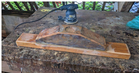
Figure 63: Mast foot glued from two pieces of lumber
