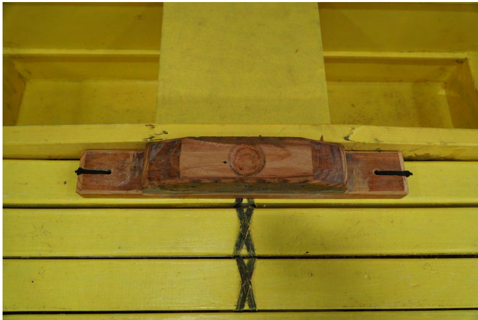
Figure 107: Mastfoot lashed on top of the deck and secured to the turtle-chest board
