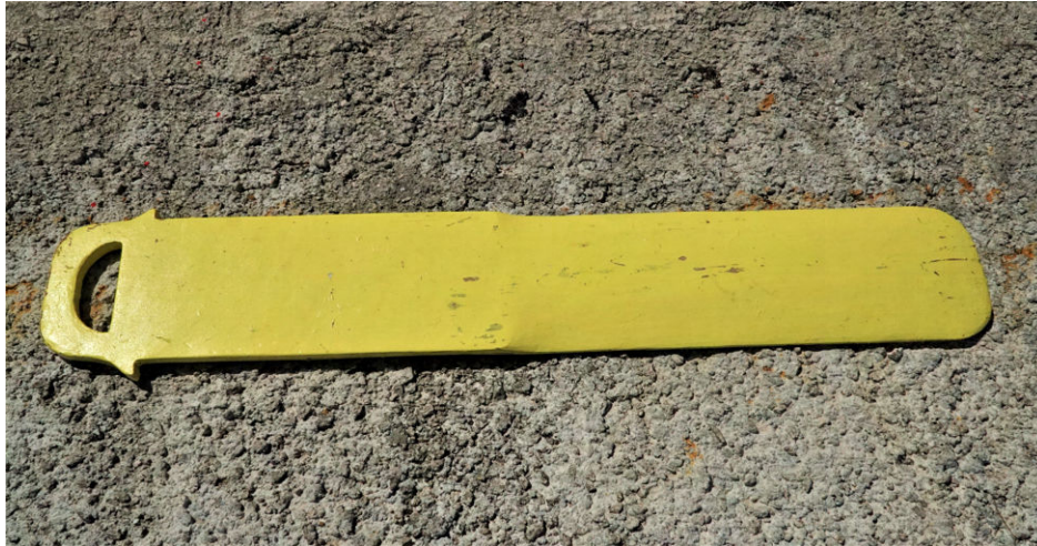
(a) Only the lower 3 ft (1 m) of the leeboards are shaped. The upper part, which always stays in the leeboard case, remains rectangular.
