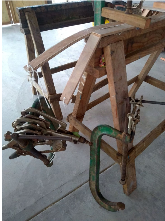
Figure 25: Sample to demonstrate the strength of glass fiber. The right (broken) strip is untreated 3/8 in (9 mm) marine plywood, the left sample is a plywood strip of the same dimensions but covered with a layer of 180 g (6 oz) glass fiber cloth on each side. The glass fiber covered sample on the left was able to carry twice the load of the right sample before the plywood in between the glass layers collapsed.
