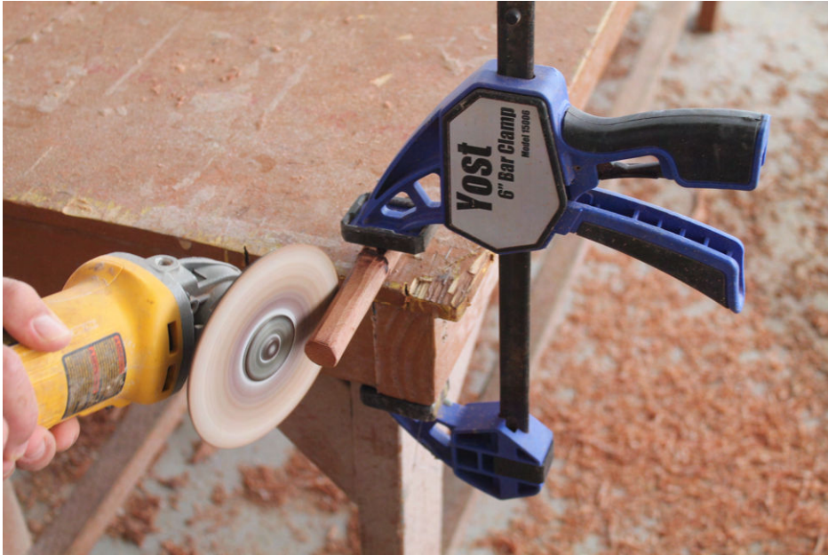
Figure 61: A hardwood dowel is cut using an angle grinder. The end of the dowel will be cut off later anyway so there is no need to shape it all the way, as long as the diameter is constant over a length of 3 in (80 mm).
