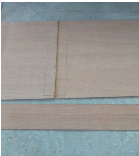
(c) The position of the doublet is marked with a pencil.
