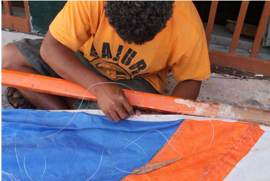
Figure 86: Lashing holes for the sail
