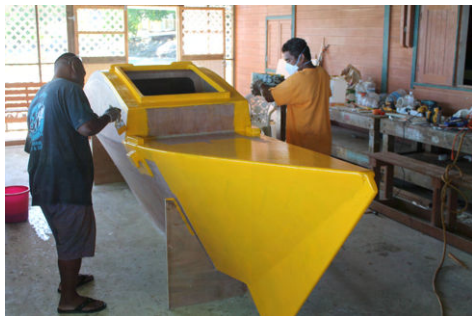
(c) The main surface is painted with the rollers.
