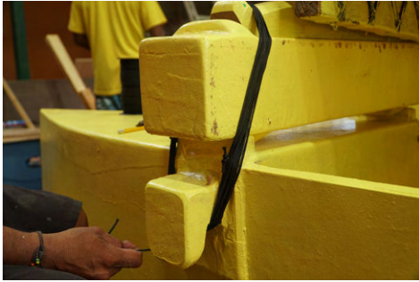
(a) Loop the lashing rope around beam and beam cleat.
