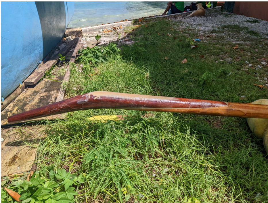
Figure 75: Hardwood mast top ( lot ) scarf-glued to the top of the mast
