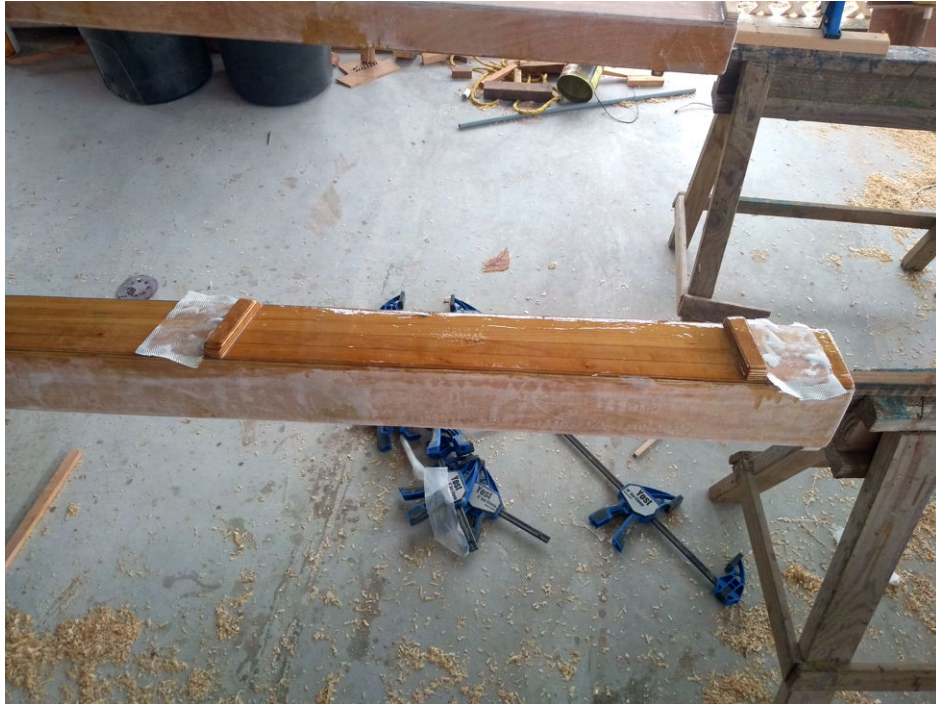
Figure 101: Alignment blocks on the bottom of the beam. The contact area of beam and beam blocks is reinforced with additional glass.
