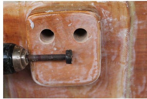
(b) Holes (at least 3/4 in) are drilled into the cleats through the cleat base in the hull. Be aware, the holes are not drilled all the way through! The inside must remain sealed! The drill is stopped 1/8 in before it breaks through on the inside. Mark the drill bit so you know the maximum depth this hole should be.
