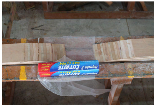
(c) Three scarf joints waiting for glue. Clamps or something heavy will be sufficient to keep them in place until the epoxy has cured. Wax paper is used to separate both joints from each other.
