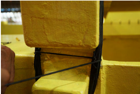
(c) The connector for the windward stay bridle is included into the beam lashing of the windward hull.
