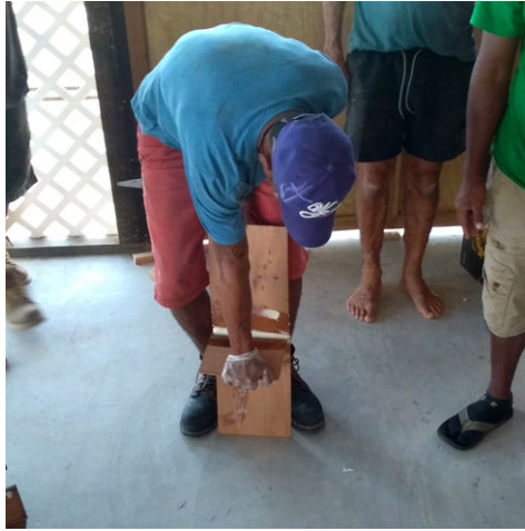
(a) Breaking test of a fillet sample
