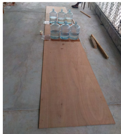
(d) The ply sheets are joined by glued on doublets. Water bottles are used as weight to keep everything in place.
