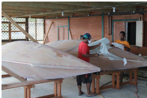
(a) Hulls turned on one side to work on a horizontal surface.
