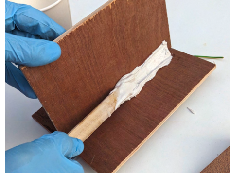
(b) The fillet mix is applied to the joint.
