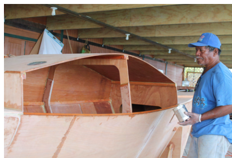
(b) Hulls are prepared with glue and resin.
