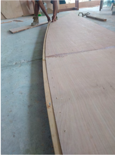
(a) Keel lumber and holes for the copper wire stitch
