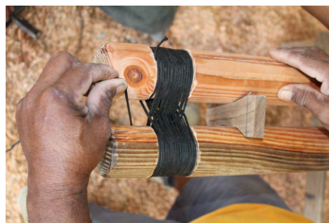
(b) Lashing fastened in a figure-eight motion
