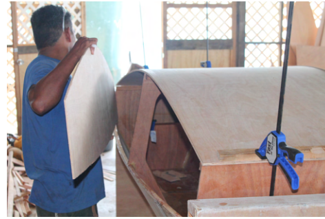
(b) Fixed by clamps, the side panels are cut according to the shape of the roof and the shear.
