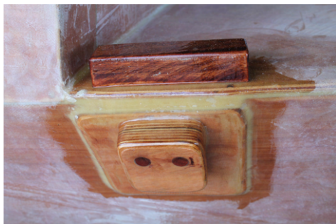
(c) The blocks should not touch the cabin bulkheads to allow water to drain.
