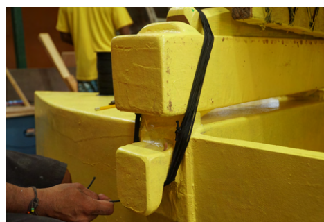
(b) Loop the lashing rope around beam and beam cleat
