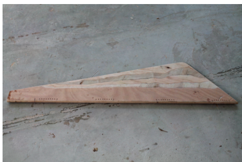
(a) Four sets of nine holes for the hinge lashings are pre-drilled with twice the required diameter.
