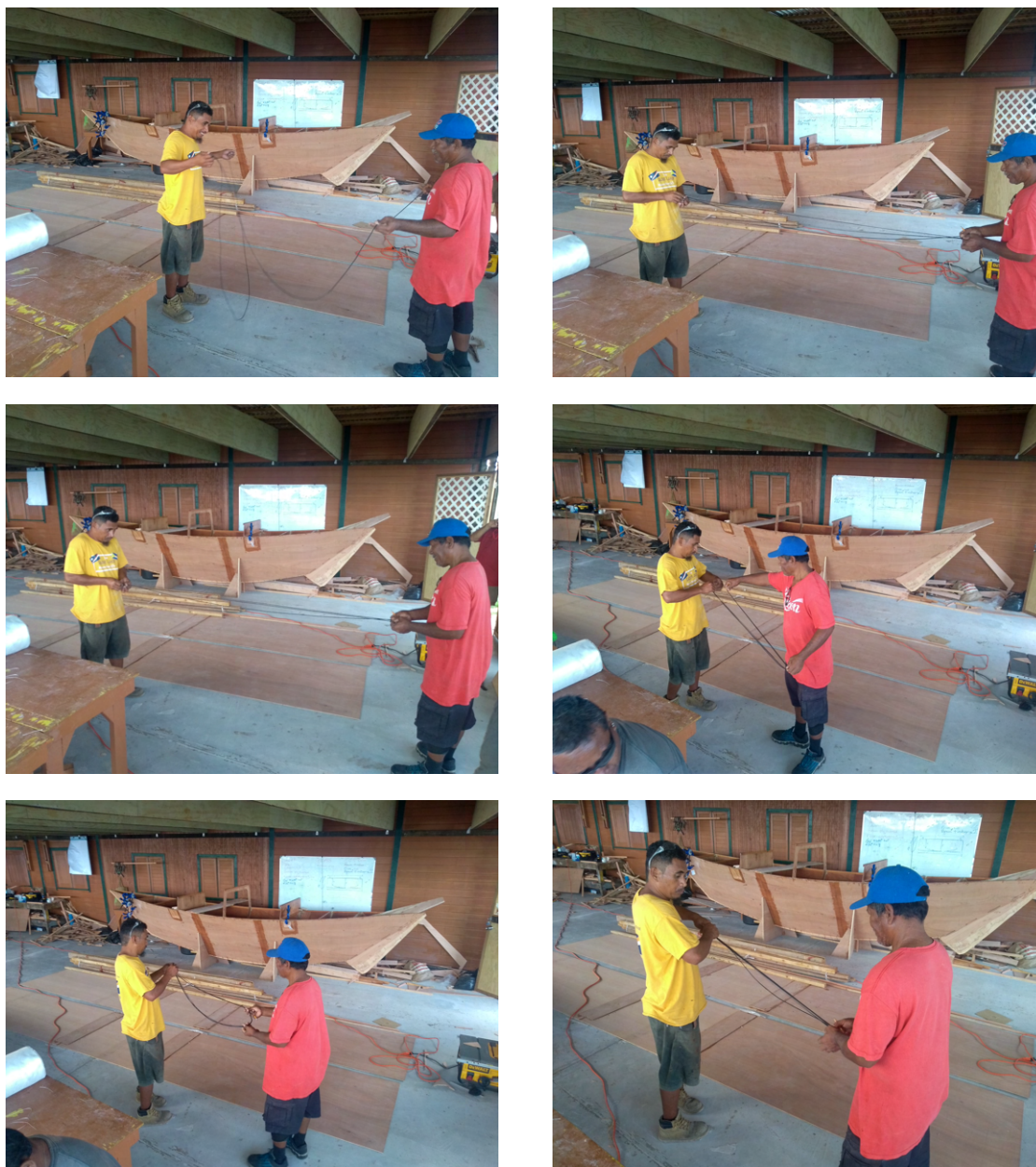
Figure 40: Preparation of the master string: It is folded to the required fraction, i.e. 1/2 , 1/3 , 1/4 , 1/6 , 1/8 and so on.
