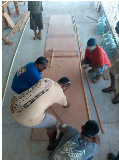
(c) The bow line is marked, as measured by the master string.
