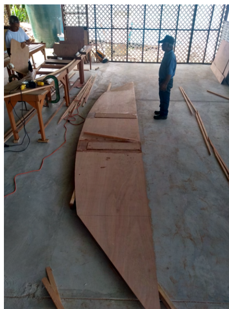
(d) The side sheet is ready to have the sheer stringer glued on.
