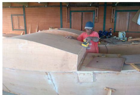
(b) All edges are rounded and filled with thickened resin (if needed).
