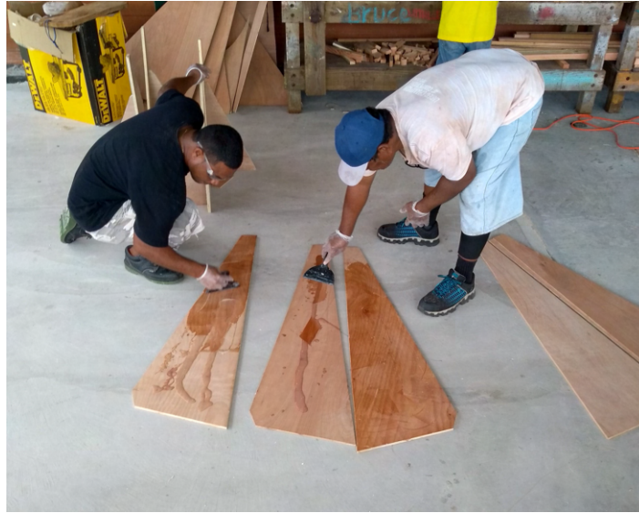
Figure 51: Each skeg is glued from two 3/8 in (9 mm) and one 1/4 in (6 mm) plywood.
