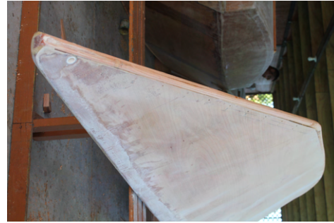
(b) The bow lumber is rounded to make it more streamlined.
