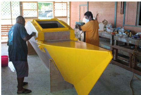
(c) The edges are carefully finished with a paint brush
