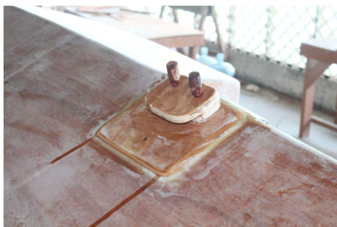
(c) Squeezing out the resin with the pins, ensures enough resin along the pin and a proper bond.
