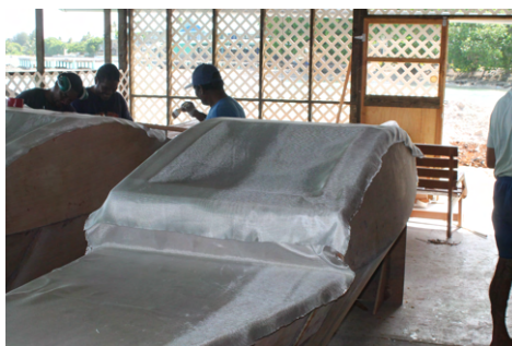
(c) Additional glass cloth is prepared for the cabin sides
