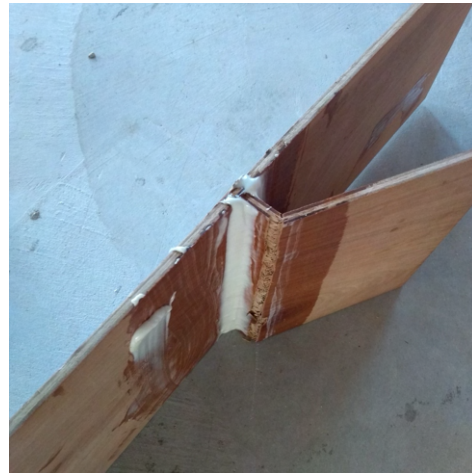
(b) Broken fillet sample: if it breaks outside the joint and the fillet remains clean and smooth, then the bond strength exceeded the material strength so the size and density are strong enough.
