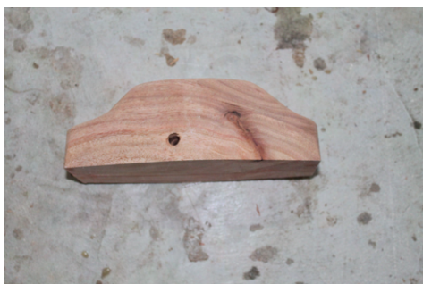
(e) Both holes are sealed with epoxy from inside.
