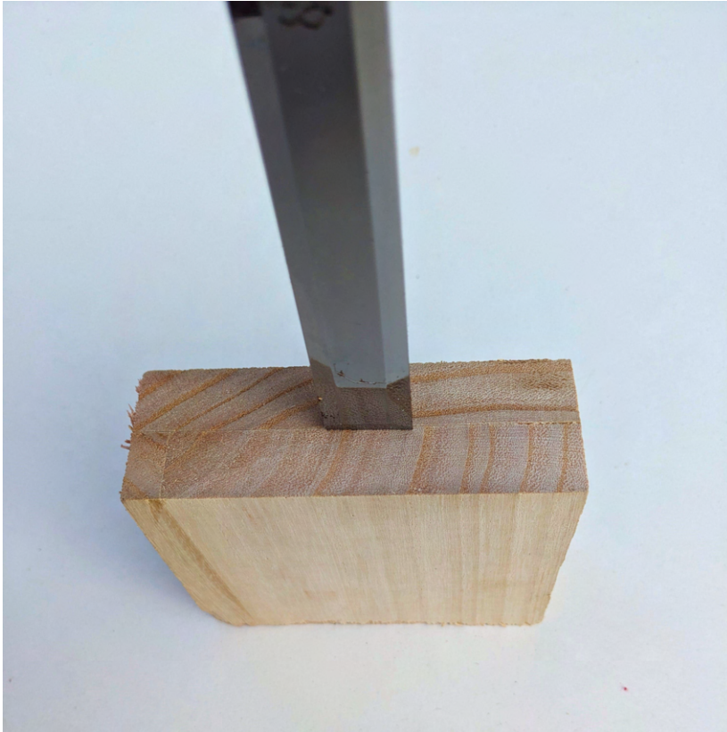
Figure 20: Breaking test for an epoxy joint. Two pieces of wood are glued together with epoxy. The chisel is placed on the glue line to split the blocks apart. The epoxy itself and its adhesion to the wood should be stronger than the wood and therefore result in the wood splitting right next to the joint.
