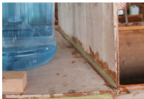
(c) Fillet between deck and cabin bulkhead
