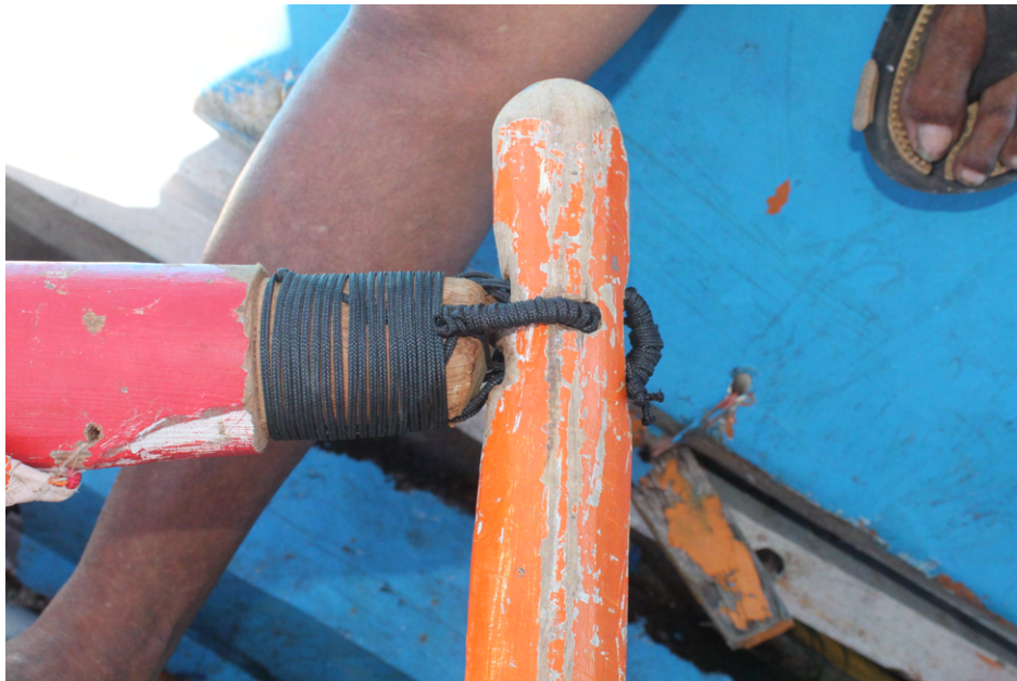
Figure 137: Lashing of the spar front ends ( kapelpel )
