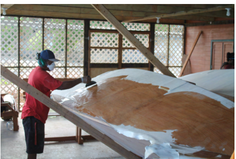
(e) There should be a three finger wide overlap at the keel and bow.
