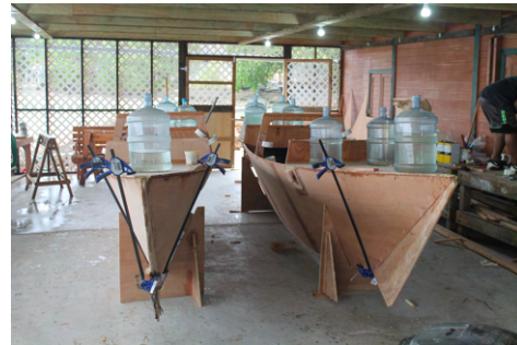
(b) It is important to use enough glue (it should squeeze out a little bit everywhere) to create a strong bond without any gaps.
