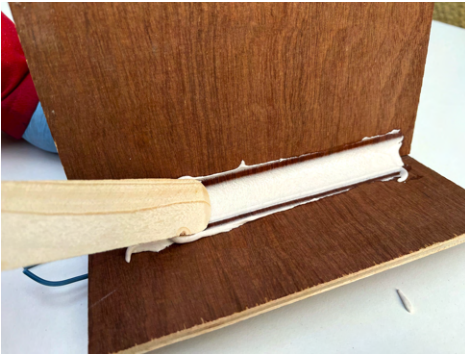
(c) A spatula with a round tip is used to create a smooth radius.
