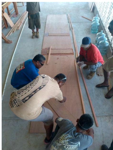
(a) The bow line is marked. It is measured by the master string.
