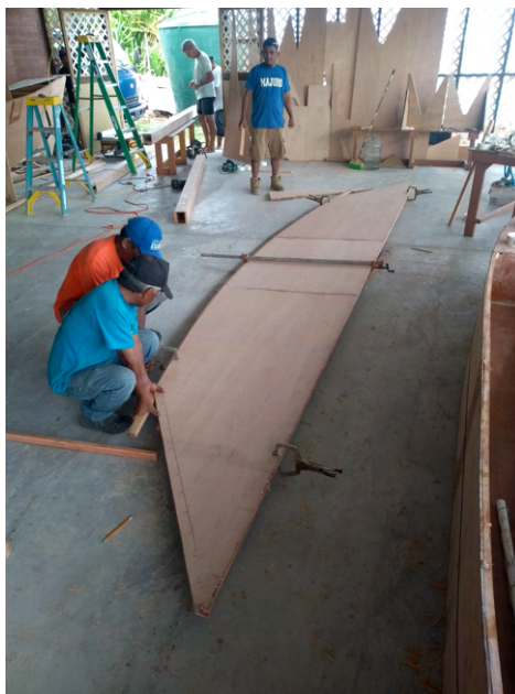
Figure 66: Assembling process of the side panels: Keel, bow and sleg are clamped in between the side panels
