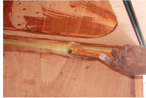
(b) The 'thickness' of the epoxy mixture is critical, especially if flour is used. A runny mixture will run off a vertical fillet leaving a weak joint.
