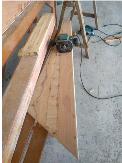
(c) The leading edge is rounded using a router (see 12 d).
