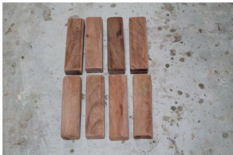
(a) Eight hardwood blocks of the same size are cut as support for the cross-beams
