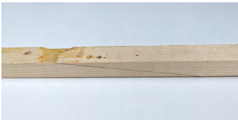
Figure 21: Scarf joint of a lumber batten (side view). The long bevels increase the bonding surface and therefore the strength of the connection.
