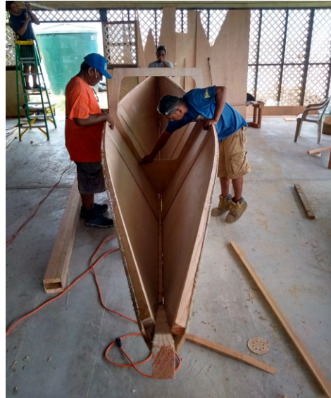
(d) The center bulkhead is locked in place. Gaps between the hull and bulkhead should be minimal.
