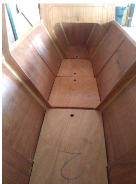
(d) The finger hole makes it easy to lift the boards and gain access to the bilge.
