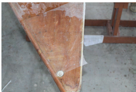
(c) The bow eyelet is reinforced with glass fiber tow. A sheet of wax paper is used to smooth the surface.
