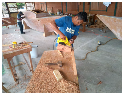
(b) The mast bases are planed and sanded smooth.
