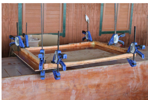
(c) The hatch cover is made from 3/8 in (9 mm) plywood and lumber from the same cross section as the hatch frame. The long pieces of lumbers are ground to fit the bent shape of the cabin roof.
