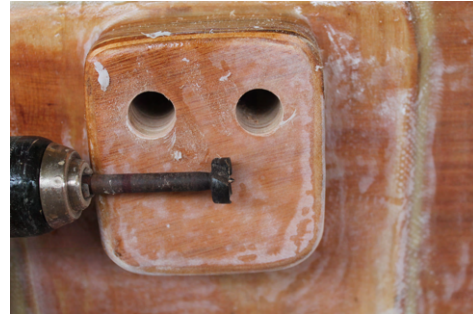
(b) Holes (at least 3/4 in or 20 mm) are drilled into the cleats through the cleat base in the hull. Be aware, the holes are not drilled all the way through! The insides must remain closed! The drill should be stopped 1/8 in (3 mm) before it breaks through on the inside. Mark the drill bit so you know the maximum depth this hole should be.
