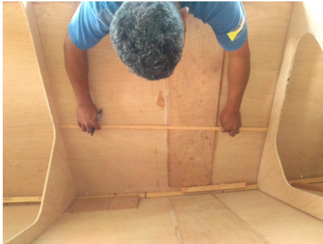
(a) Measuring the individual lengths for the support stringers and marking their position on the hull
