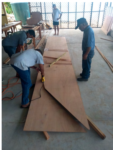
(c) The side sheet is cut out using a jigsaw.
