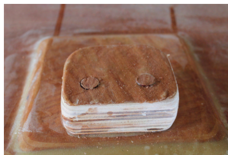
(d) After the glue is cured the pins are trimmed and sanded.
