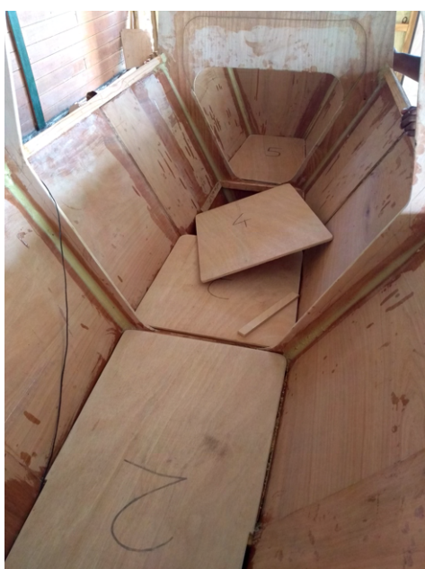
(c) Finished bunk-boards in the hull
