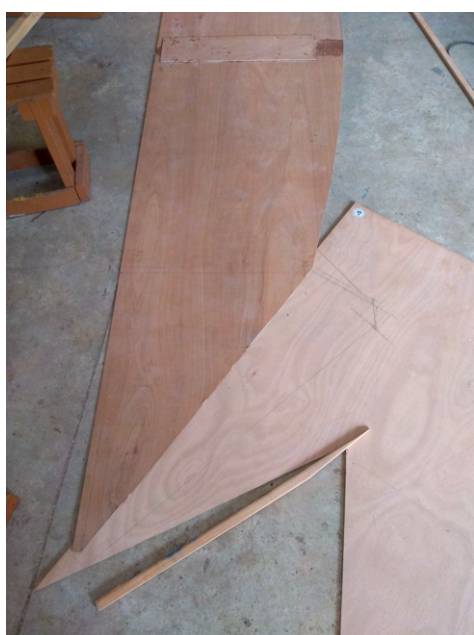
(a) The skeg's dimensions are determined by placing a plywood sheet underneath the hull side panel.
