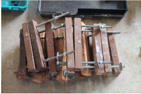
(a) DIY wood clamps (20 pieces, used for beams only)
