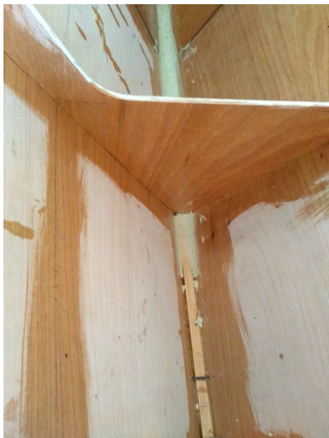
(a) Keel fillet under construction
