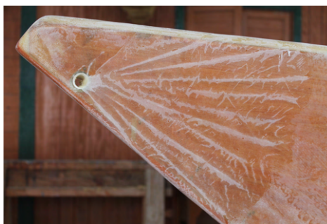
(d) The star shape (to spread the load across a larger surface) of the glass tow is clearly visible after sanding.
