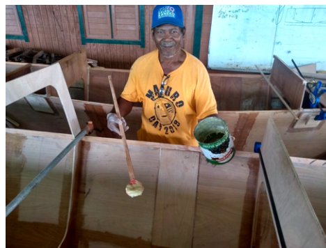
(b) Tools with long handles might be helpful for the deep keel fillet.
