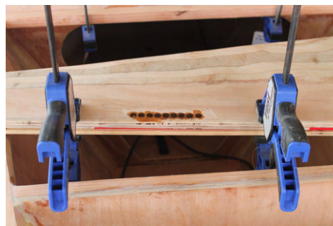
(b) The bottom of the holes are closed with duct-tape (red) and further sealed by a stick clamped underneath.
