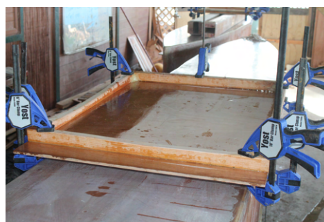
(d) The front of the hatch cover plywood extends approx. 3 fingers (2 in/50 mm) beyond the front lumber to allow space for the holes of the rope hinge (see 6.9). The holes are pre-drilled, filled with epoxy and drilled again.
