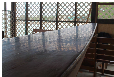
(b) The flow coat is clearly visible by the absence of any fiber structure of the glass cloth. The surface is shiny.
