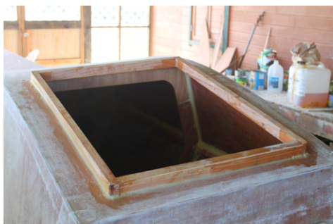
(a) The hatch frame is made from 1 x 2 in (25 x 50 mm) lumber. The short pieces (bow and stern) are glued on top of the cabin roof, the long ones in the hatch opening (touching the cabin roof in a butt-joint manner).
