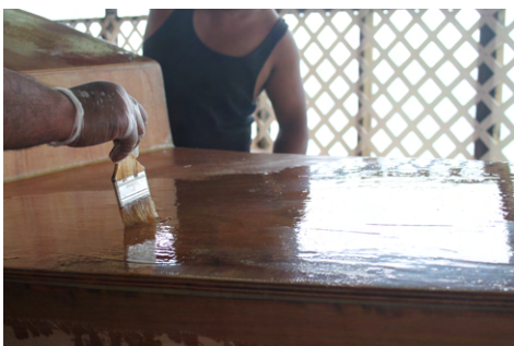
(c) Application of the flow-coat.
