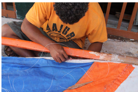
(a) The sail is stitched to the spars with 30-lb fishing line.
