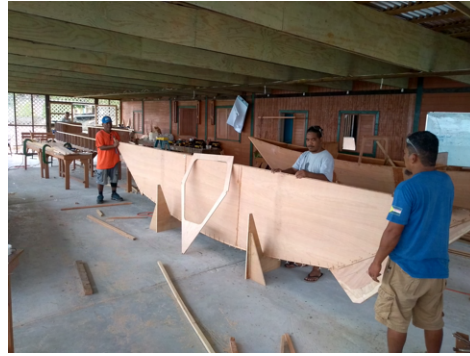
(b) Ready to spread the hull: The prepared center bulkhead is ready to grab.
