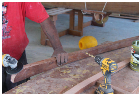
(a) Shaping of the keel shoes, from local hardwood, according to the shape of the keel.
