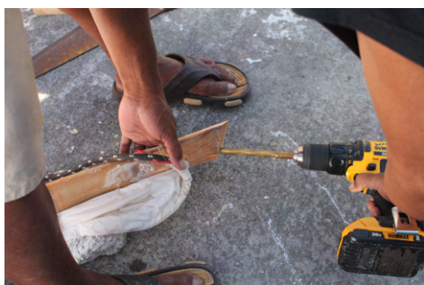
(c) A hole for the leech line is drilled into the end of the spar.
