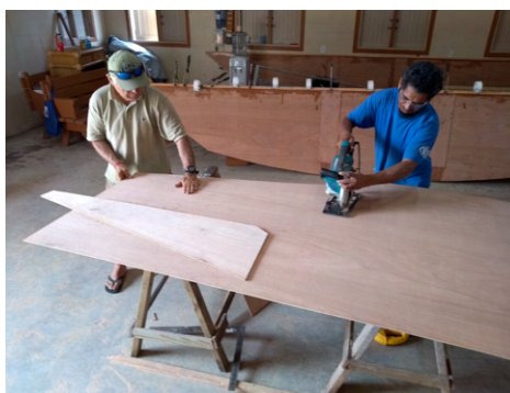
(b) The first plywood skeg is used as pattern to cut five more pieces (three for each hull).
