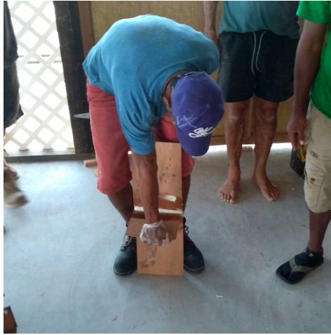
(a) Breaking test of a fillet sample
