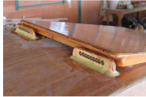
(b) Hinge plate holes match up with the hinge holes of the hatch cover.
