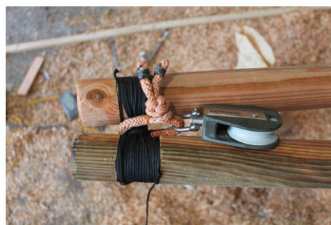
(d) Finished mast head lashing with halyard pulley
