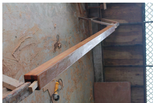
(b) Beam after flow coat with epoxy resin
