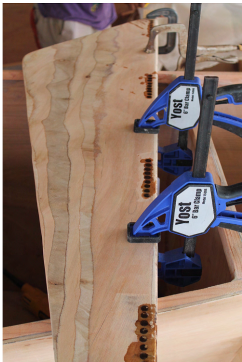
(a) The pre-drilled holes in the skeg and the rudder are filled with unthickened epoxy resin.
