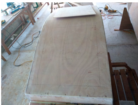
(b) The cutout for the hatch is marked on the roof.
