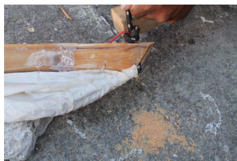
(d) The leech line is locked in the hole with a knot. The tension of the leech line is important for the sails trim and therefore occasionally adjusted.
