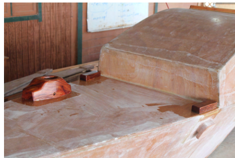
(b) The blocks are glued at the position of the beams - right in front of the cabin bulkheads and above the beam cleats. The mast feet are placed right on top of the second bulkhead. The exact position of the bulkhead is determined by knocking on the deck and listening for the change of sound of the knocks (you will hear the sound of where it is less hollow above the bulkhead).
