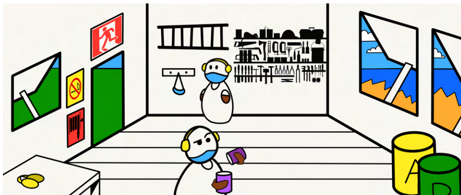
Figure 28: Establish good practices in the workshop: make sure personal protective equipment (PPE) is used and the workshop is properly set up. The workshop should be ventilated and escape routes should be known, marked and unblocked. A first aid kit, fire extinguisher and freshwater should also be on site.
