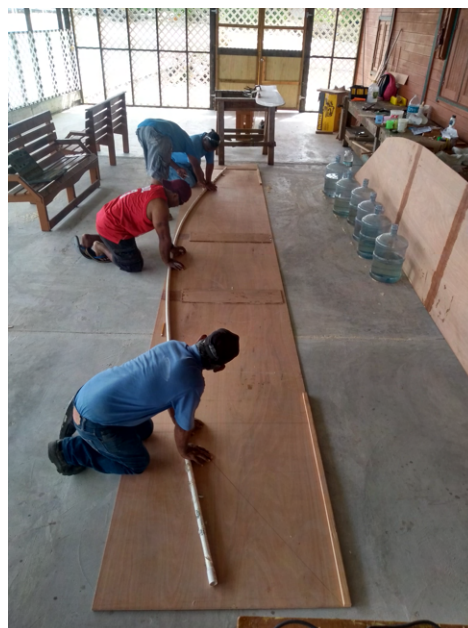
(b) The keel line is marked using a PVC pipe.
