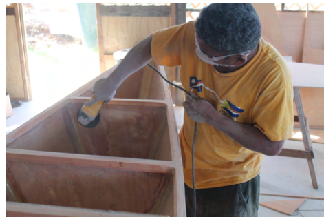
(b) The sheer and the bulkhead tops are sanded down to allow a smooth fit of the deck panels. A smooth fit is important for a strong bond.
