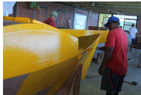
(d) The main surface is painted using rollers
