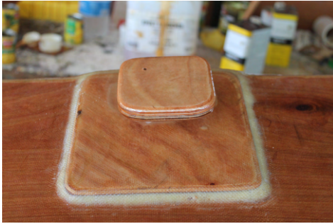
(a) Beam cleat glued outside on the reinforcement doublet on the hull.
