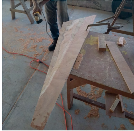
(b) The job is finished fast by using an angle grinder. The parallel lines of the individual veneer layers of the plywood give a good visual feedback on how well the rudder has been shaped.
