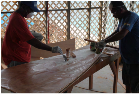
(a) The deck panels are glassed from the inside.
