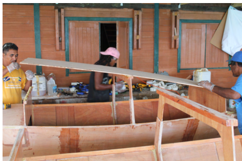
(c) The roof is placed on top of the bulkheads.
