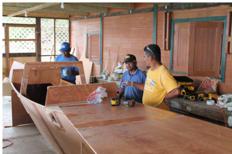
(a) Cabin sides are sanded at the bonding points
