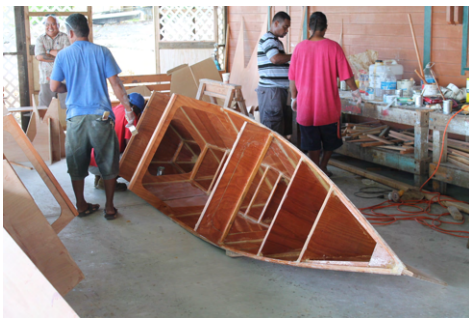
(c) The accessibility proved to be best with the hulls flipped on one side.
