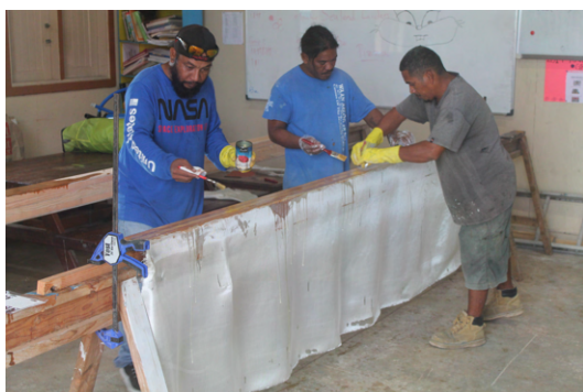
(a) Beam is glassed with a 3 ft (1 m) wide piece of 7 oz. (200 g) glass cloth
