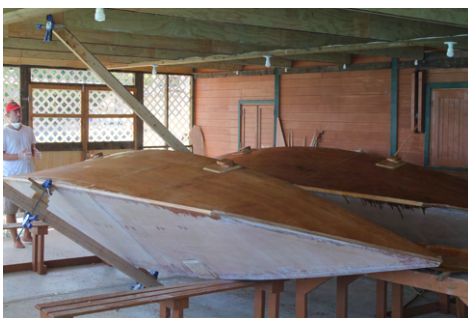
(f) First side is glassed. The second side is glassed in the same way.
