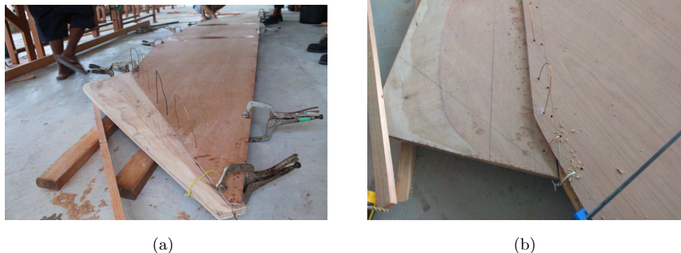
Figure 68: Integration of the skeg into the hull
