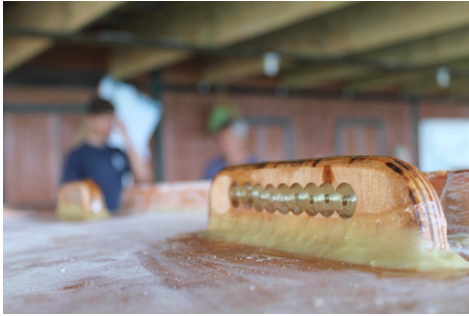
(a) Hinge plate - pre-manufactured and glued on the cabin roof with fillets.
