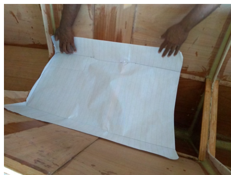
(b) The paper is pressed into the hull the same way as the bunk-board will go in later. A second pair of hands is helpful to keep the paper tight while the outline is marked.
