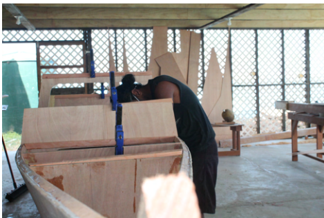
(a) The top edges of all bulkheads are fitted with 1 x 1 in (25 x 25 mm) lumber to increase the bonding surface for a strong joint with the deck and the cabin roof.
