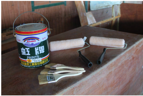
(a) Painting equipment: regular exterior house paint, brushes and big rollers
