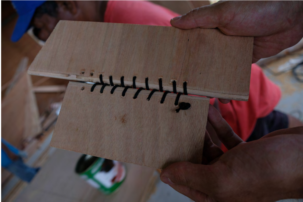
Figure 27: Functional model of a hinge lashing
