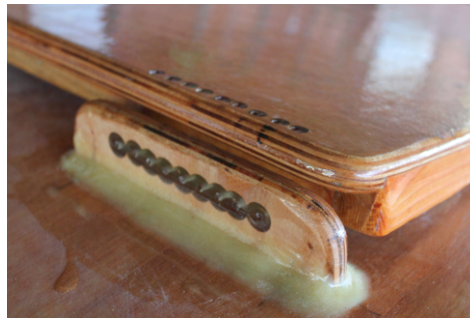
(c) The hinge plates and the hatch cover should almost touch each other.
