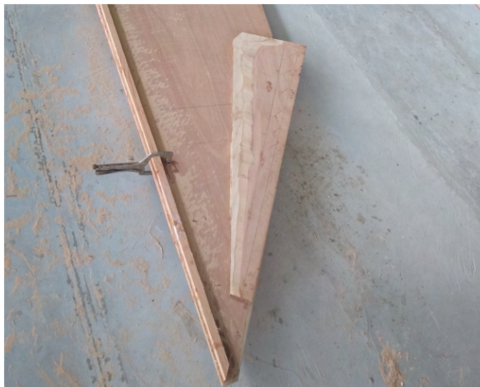
Figure 52: Skeg with tapered trailing edge
