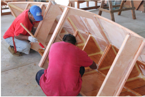
(a) Application of epoxy inside the hull.
