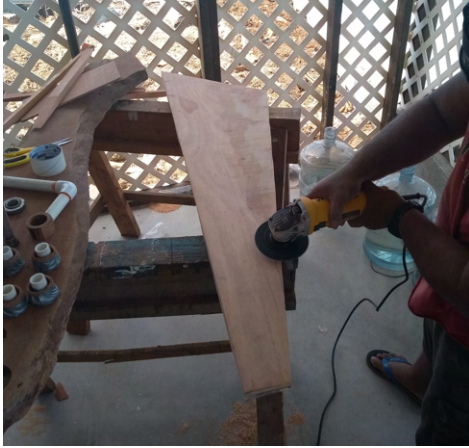
(a) The rudder is glued from two pieces of 9 mm (3/8 in) plywood and tapered at the trailing edge to 3 mm (1/8 in) to create an airfoil shape.
