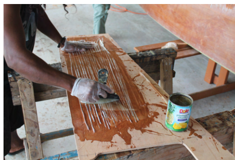
(b) Tow wet out with epoxy resin
