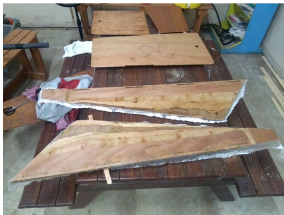
Figure 86: Glass the rudders with 3 layers of 7 oz. (200 g) fiberglass cloth.
