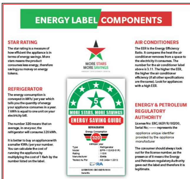
Figure 26: Sample energy efficiency label in Kenya (EPRA)
