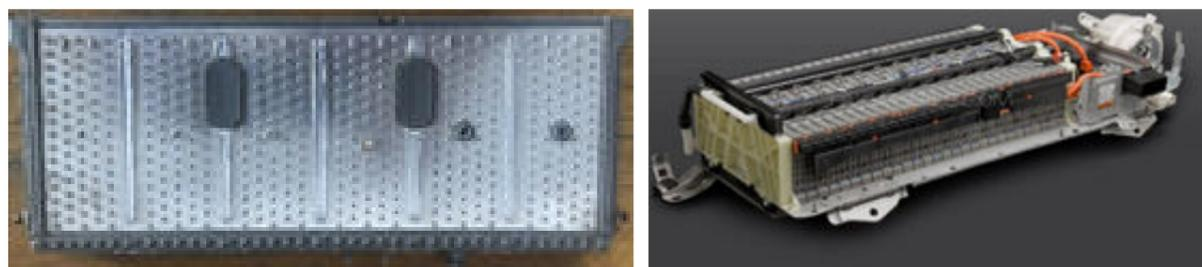
**Figure 3:** Module of nickel metal hydride battery (left) and battery pack of a Toyota Prius generation 2 (right)
