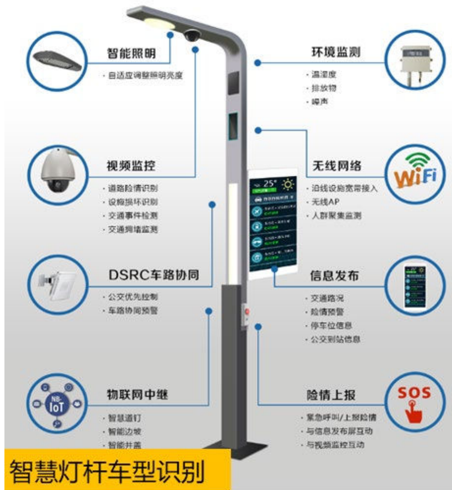
Figure 13: Example of smart lamp posts with vehicle recognition device (Source: SUTPC)
